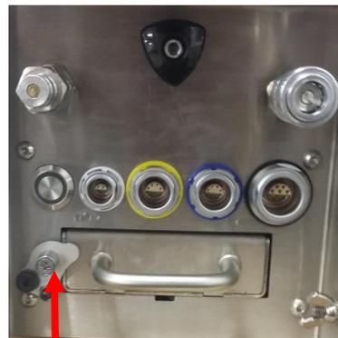
This mechanical lock device holds the battery firmly in place, and prevents accidental disconnection.
