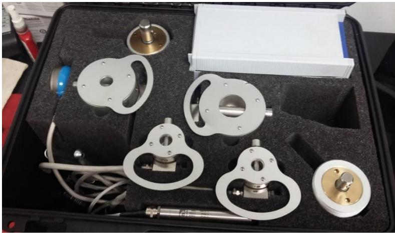
Figure 5.1 – Load cell assembly case
