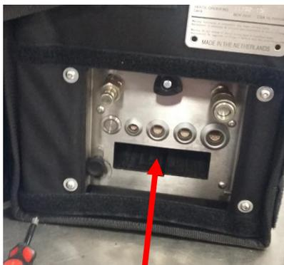
The Hand Pump Case Battery receptacle is located on the interface panel, which is on the side panel of the Hand Pump case.
