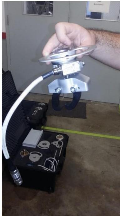
Figure 7.1 – Example of Load Cell mounted to Load Cell Claw Assembly
